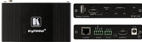
FC-18 is a display ON/OFF controller for 4K@60Hz (4:4:4) HDR HDMI signals. It accepts and outputs an HDMI signal after reclocking and equalizing. On detection of the onset of an input signal FC-18 sends an ON command to the display or projector and on detection of the loss of the input signal FC-18 sends an OFF command. FC-18 can also be used to control a display device manually via front panel buttons, Ethernet or contact closure switches
